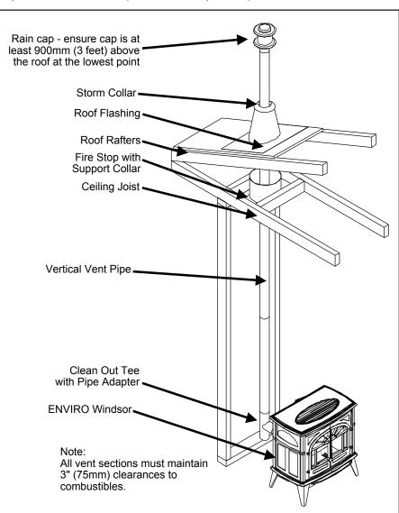
Figure 13: Inside Vertical Installation.
